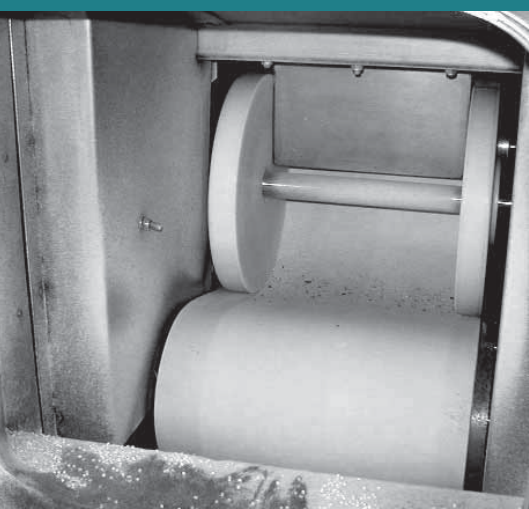
Throwing Belt A robust endless rubber belt is rotated at high speed to ensure reliable high capacity product loading
