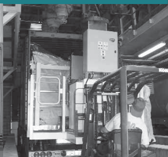
Operation 3 ❖ The CLS is mounted on the container
