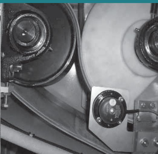
Safe Operation The belt is automatically monitored for misalignment or slippage during operation to ensure safe operation
