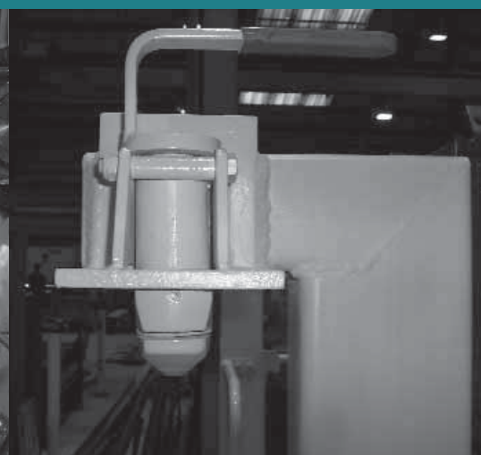
Simple Mounting The CLS is firmly secured to the standard ISO container mounting lugs by simple twist lock fixings
