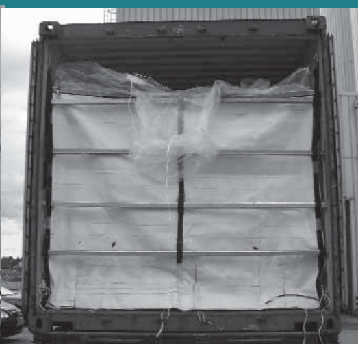
Operation 2 ❖ Container with empty liner fitted
